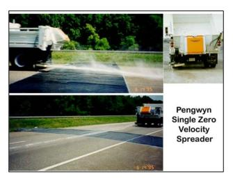
material distribution to the lane of application. ODOT has used zero velocity spreader systems in the past, but due to their increased maintenance costs and high failure rate, most systems have been removed and are no longer in use.
