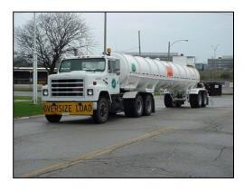
Additionally, ODOT has trucks equipped with Direct Application Wetting Systems capable of applying large quantities of brine directly to the road surface. These systems apply brine prior to an event preventing snow and ice from bonding to the pavement (anti-icing) or during light events removing smaller quantities of snow and ice (deicing). ODOT utilizes both removable and dedicated direct application systems. The removable systems have tanks
