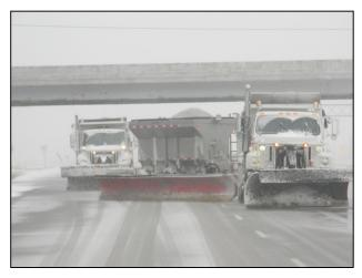
a six ton capacity hopper and material spreader. However, a wetting system and liquid storage tank can be added. Although modified, the existing hydraulic controller operates the plow including swinging the plow to the right and left, lowering and raising the plow blade, and controlling the material output of the spreader. At the conclusion of this winter's testing period, ODOT will evaluate the results and consider adding the Tow Plow to the snow removal fleet.
